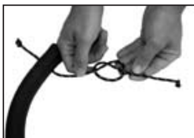
You can tie further knots in the leader lines for tuning purposes. Start with knots an equal distance apart, you can always adjust them later to suit.
