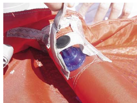
6. Fasten the velcro over the valve. This secures the valve in place.
