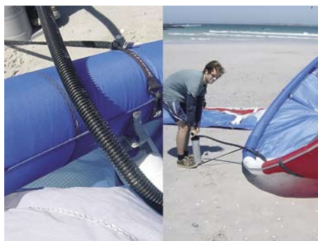
8. Connect the pump leash to the kite, turn the kite so it is downwind and inflate the LE tube.
