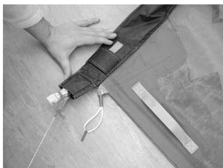
Lay the kite on its back with ribs facing up. Ensure the leading edge bladder and all ribs are deflated. When repairing the leading edge tube, open the end flap by pulling back the Velcro from under the securing loop.
