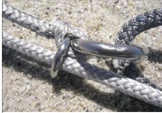
Fig. 5 Thread 5 th line through stainless steel guide ring at the top of the depower system
